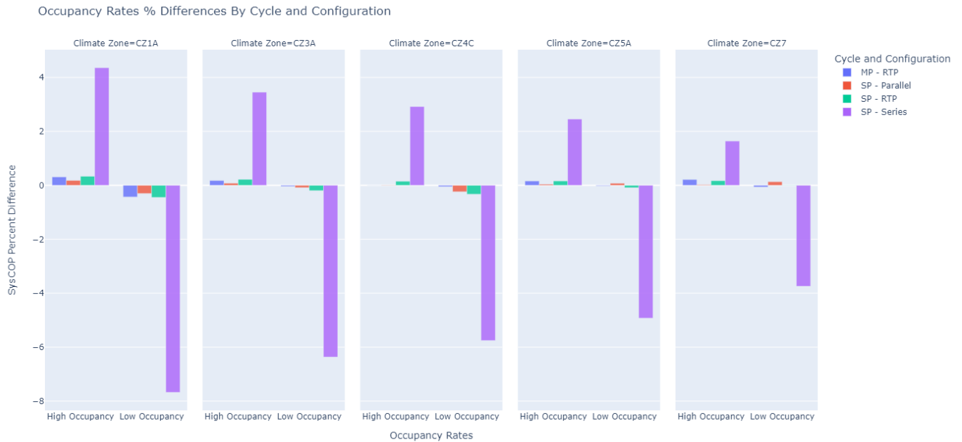
Figure 7. Percent Difference in SysCOP for Different Building Occupancy Rates
