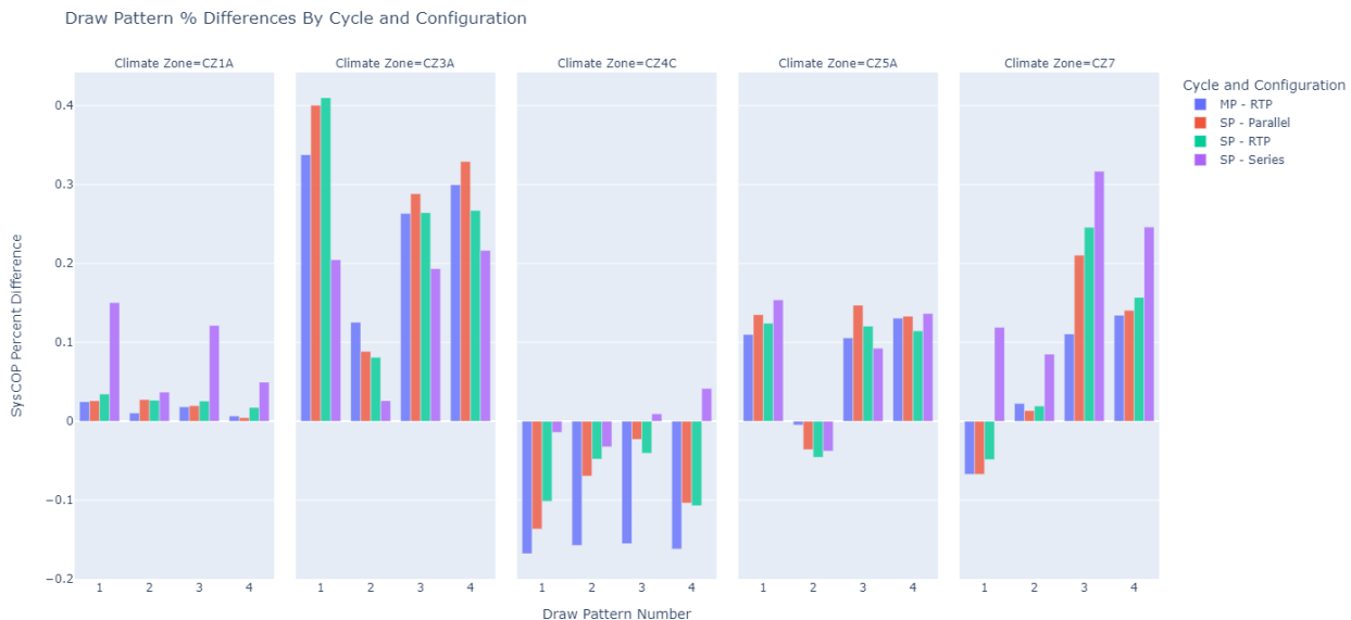
Figure 8. Percent Difference in SysCOP for Different Draw Pattern Shuffles
