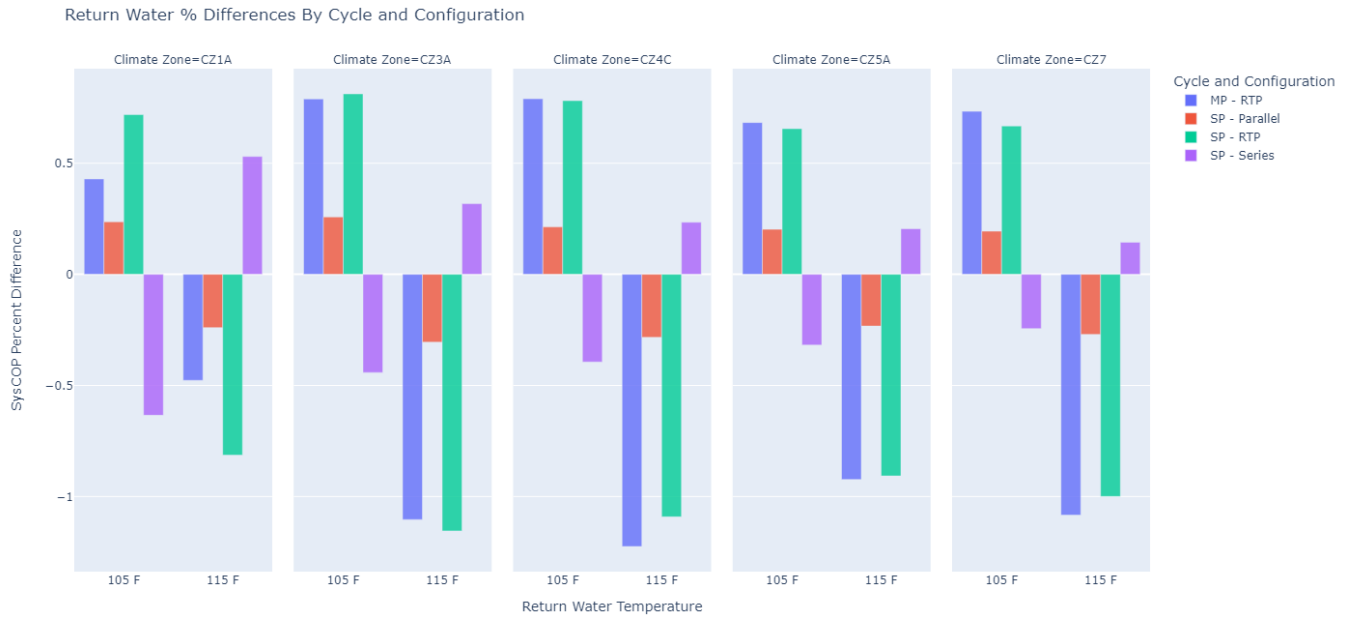
Figure 5. Percent Difference in SysCOP for Different Return Water Temperatures
