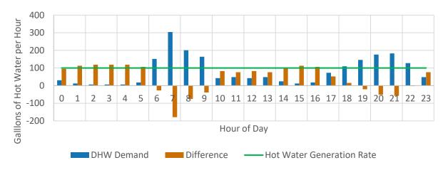
Figure 7. Hot water (HW) use, heating rate and difference throughout the day.
