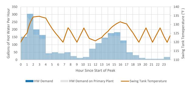
Figure 9. Swing tank simulation plot.
