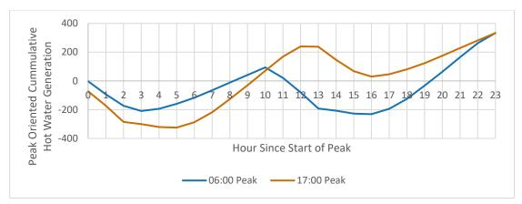
Figure 12. The cumulative supply after peak events for a load shift scenario.
