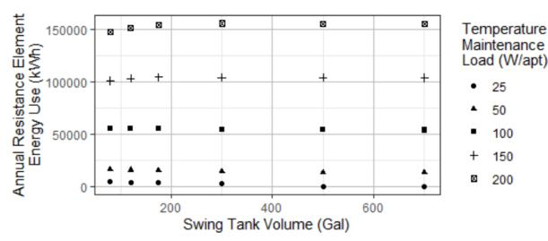
Figure 13. Annual energy use in the swing tank with swing tank volume for different temperature maintenance loads.
