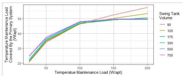
Figure 15. Annual temperature maintenance load covered by the primary system for the modeled temperature maintenance loads.
