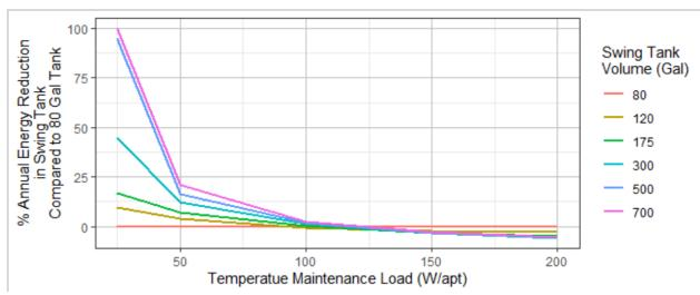
Figure 14. Percent of energy reduction in swing tank from increasing the tank volume above 80 gallons as a function of the temperature maintenance load (For a building with 118 dwelling units).
