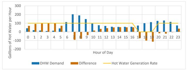
Figure 11. A load shift scenario where the systems is HPWH is excluded from 1700 to 2000.
